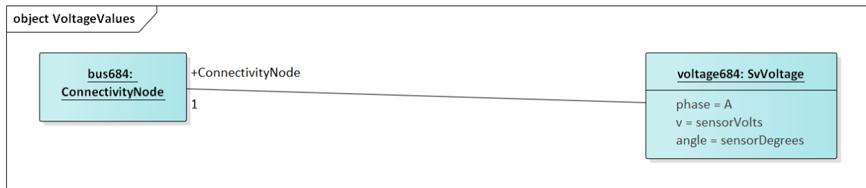
Figure 36: In this profile, a solved voltage value attaches to ConnectivityNode in GridAPPS-D. Positive sequence or phase A is implied, unless the phase attribute is specified.
